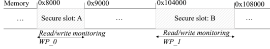
Figure 1: Sparse slot allocation limits the number of creatable secure slots to be equal to the number of available watchpoints.
