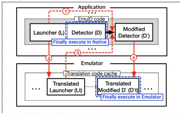
**Fig. 4.** EmuID overview. In the native environment, ① L modifies D to D'. As a result, D' should be executed, but D is executed due to cache incoherency. In the emulation environment, ② L is translated to L<sub>T</sub> in translation code cache by emulation engine. ③ L<sub>T</sub> modifies D to D'. ④ D' is translated to D'<sub>T</sub> in translation code cache by emulation engine. As a result, D'<sub>T</sub> is executed as expected.
