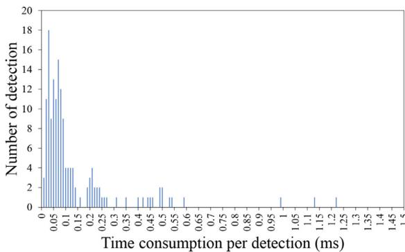
**Fig. 11.** Time consumption for detection on 155 real android devices of Amazon Device Farm. The average time to detect is 0.14 ms. The shortest time is 0.012 ms, and the longest time is 1.224 ms.
