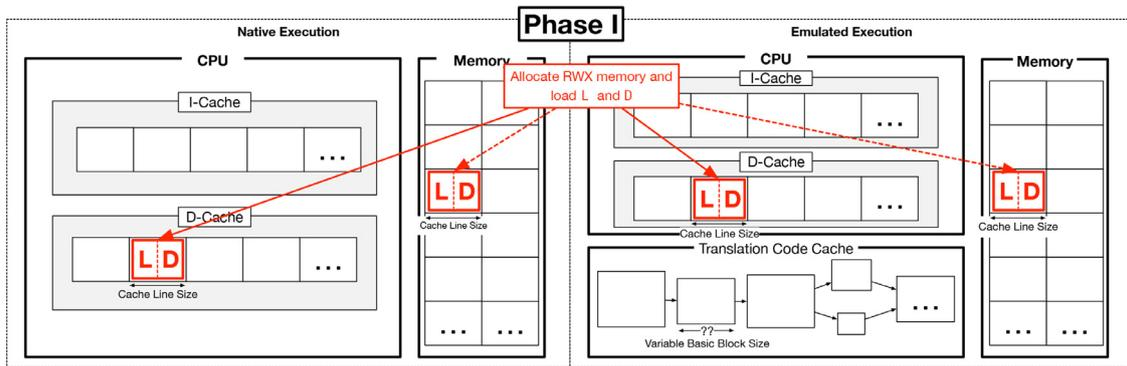
Fig. 5. Phase I. Initial State. L and D are loaded into RWX memory. To this end, L and D are first loaded in D-cache and then updated in memory.
