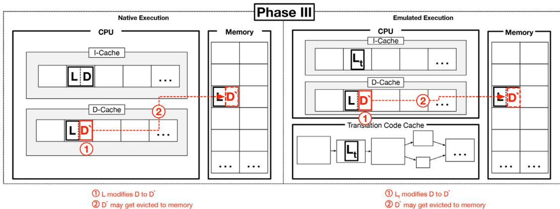
Fig. 7. Phase 3. Launcher has finished executing. The D is modified to the  $D'$ . In A, since there has been no explicit I-cache invalidation, D in I-cache is stale from this point on.
