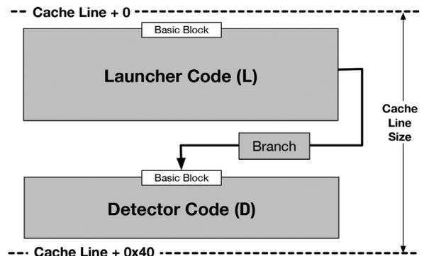
Fig. 3. EmuID Code Structure. The code is deliberately configured to have the Launcher (L) and Detector (D) that are located in different basic blocks but are loaded into the same cache line. This particular structure triggers different cache behaviors in native and emulated execution environments.
