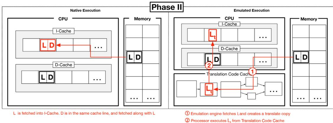
Fig. 6. Phase 2. Launcher is ready to be executed. In A, L is loaded into I-Cache. Since L and D are in the same cache line, D is loaded along with L as a side effect. In B,  $L_T$  is fetched, translated to become  $L_T$ , which is then placed in the code cache.  $L_T$  is loaded into I-cache (Notice that D is not loaded into I-cache).
