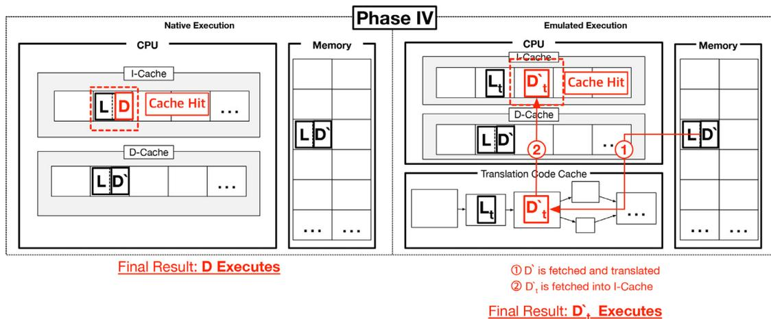
**Fig. 8.** Phase 4. D' is ready to be executed. In A, the processor tries to execute D', finds its address in I-cache (cache hit). Not knowing that D in I-cache is stale, the processor executes it. In B, the emulation engine has never executed D, and it is not found in the translation code cache (TCC miss). The code cache for D must be created. Thus, the resulting code cache in the translation code cache would be D't. And then, D't is executed on the processor.
