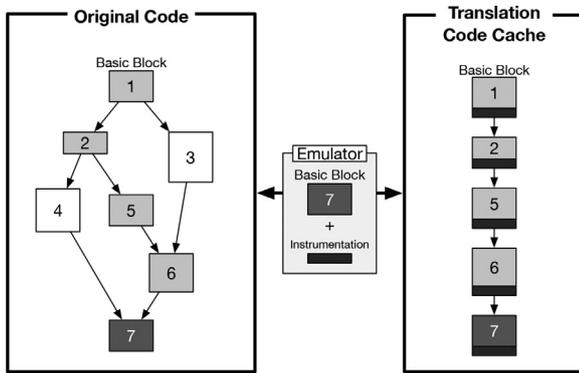
**Fig. 1.** Translation process in emulation. During the translation process, the original binary and the emulation code for one basic block are loaded into the translation code cache and then executed. After executing one basic block in the code cache, the emulation environment repeats the above process for the next basic block. The example figure shows that basic block 7 is converted and executed after basic blocks 1, 2, 5, and 6 executes.
